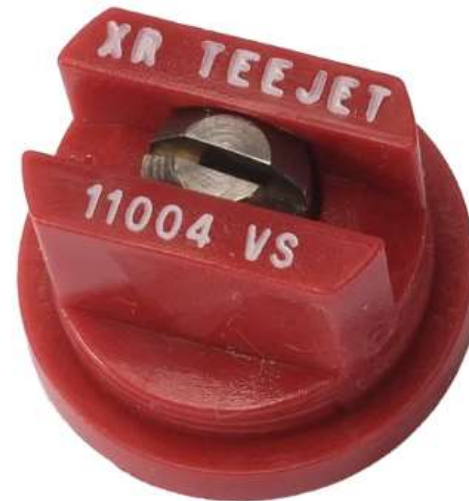
110-degree spray angle 0.4 GPM (Gallons per Minute) at 40 psi
