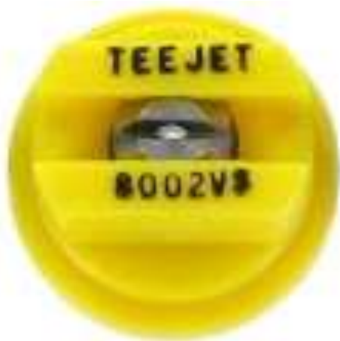
80-degree spray angle 0.2 GPM (Gallons per Minute) at 40 psi
