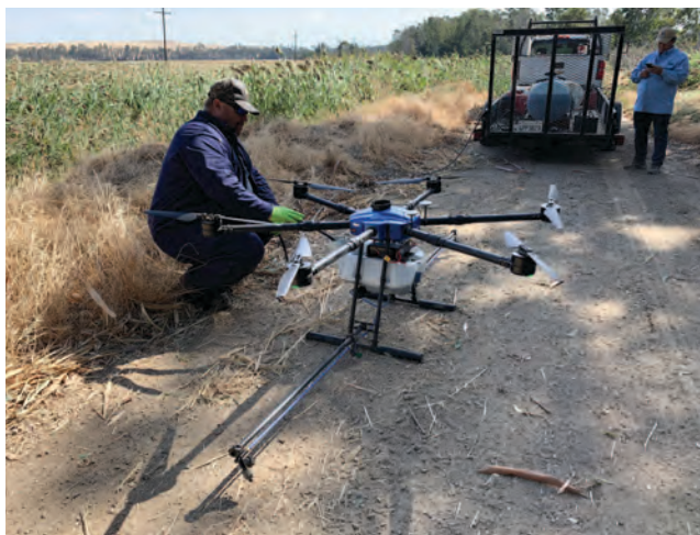
The six-rotor drone carries 3.5 gallons of herbicide. Each set of batteries powers a 14-minute flight. All photos courtesy of authors.
