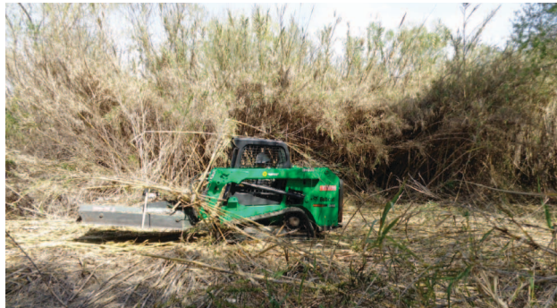
Rotary mower employed used to reduce biomass of two half-acre Arundo stands.
