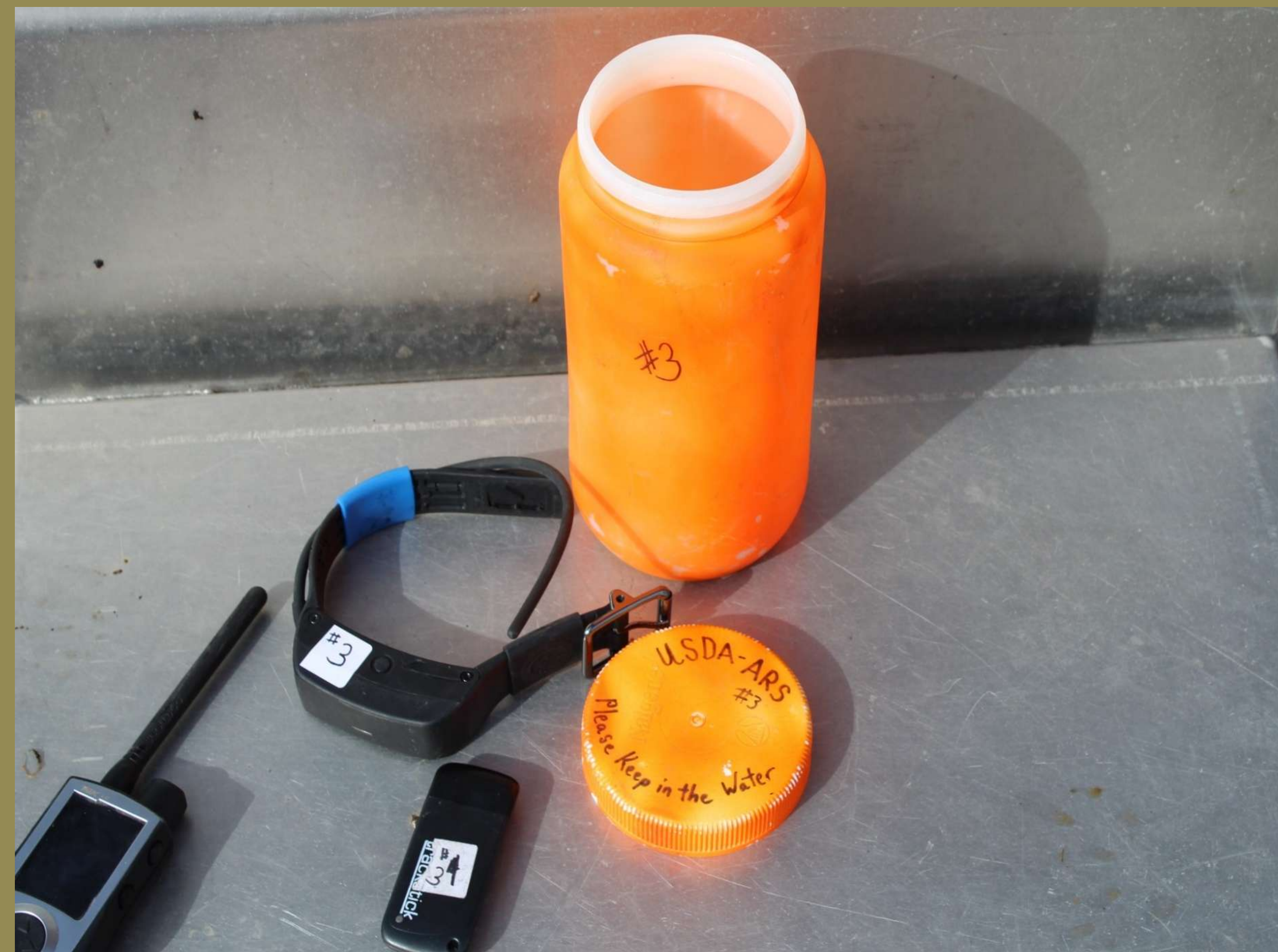
Figure 5. Setting up a bottle with radio collar and GPS recording device. The receiver for the radio collar is on the left.
