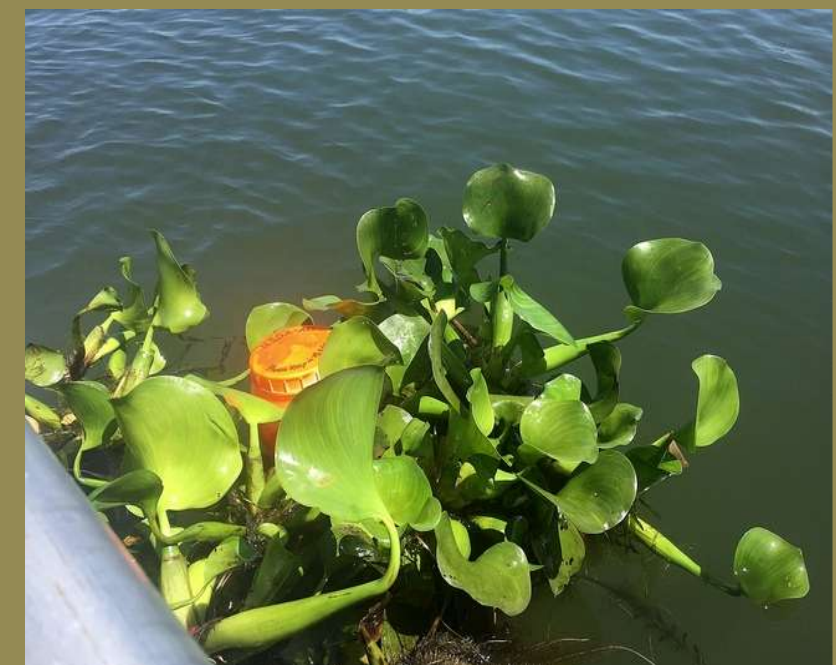
Figure 8. 4ft 2 waterhyacinth mat with GPS tracker after drifting for 3 hours Sacramento-San Joaquin Delta, CA.
