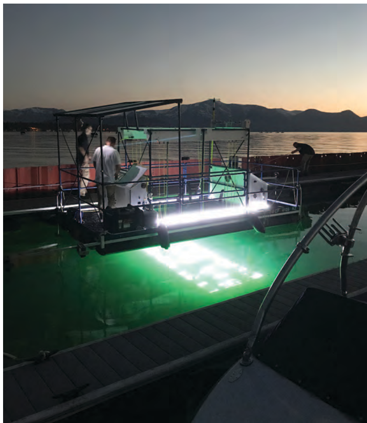
Field tests of the ultraviolet-C (UVC) light rig used to treat invasive plants.
