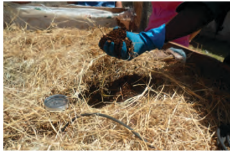
A worker measures both temperature and oxygen at a typical static compost pile. The thermometer is visible. The cables in the foreground are connected to the oxygen sensor inside the compost pile. Photo courtesy of the Sustainable Sanitation Alliance
