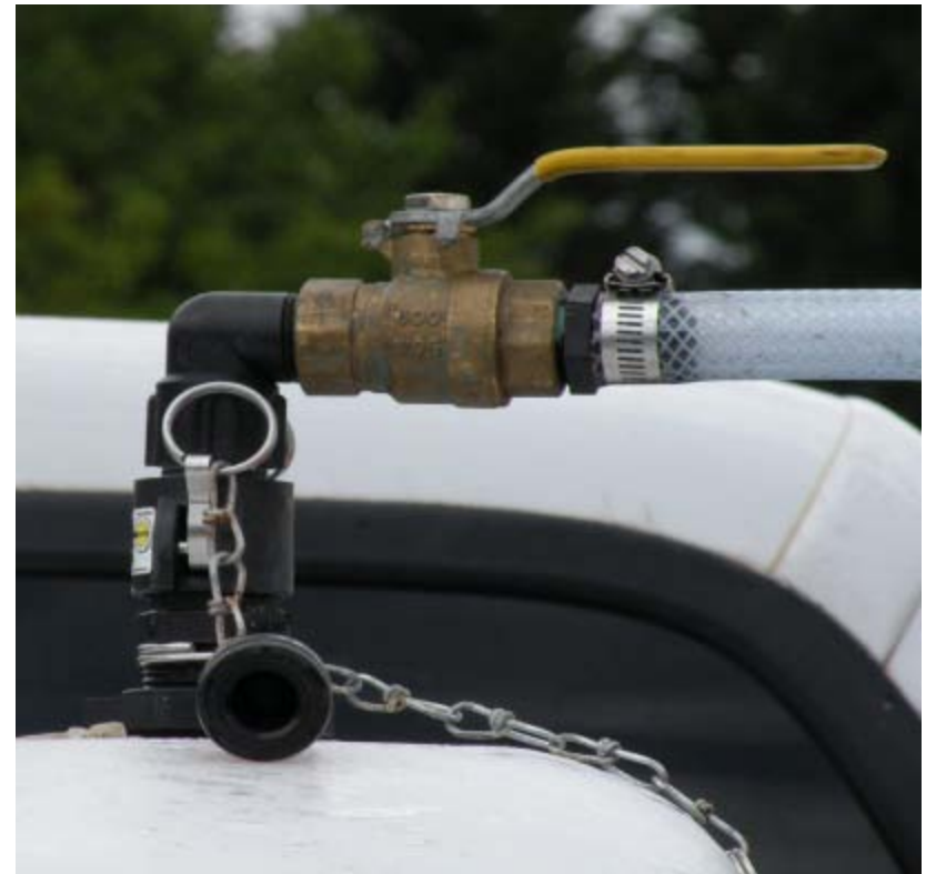
Camlock valve connection to spray tank
