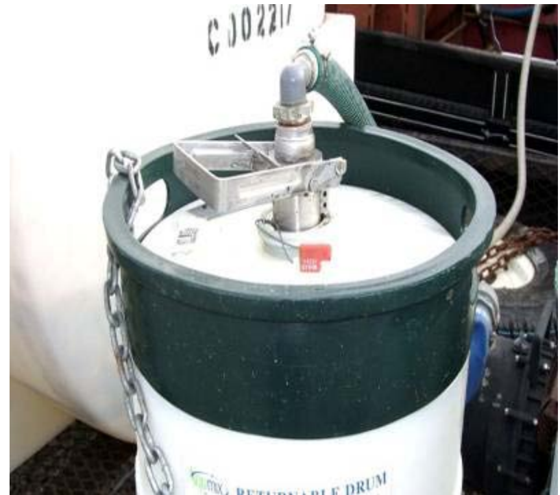
Micromatic™ vented valve coupler on supply container
