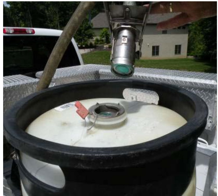
Micromatic™ valve connection to Supply Container
