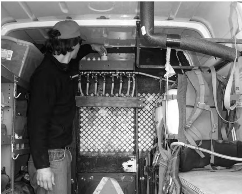
**Mark at the manifold** where valves are calibrated for each herbicide. The water reservoir is mounted at right, behind backpack sprayer.
