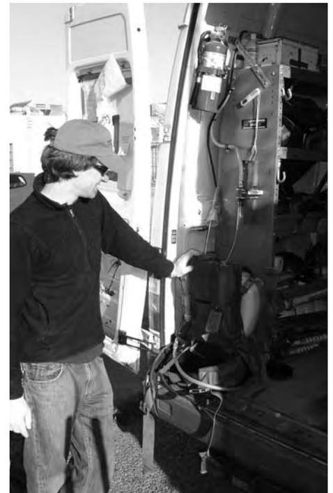
**Backpack sprayers** are filled at the rear bumper. The system takes about a minute to fill a backpack sprayer, with no handling of herbicide containers.
