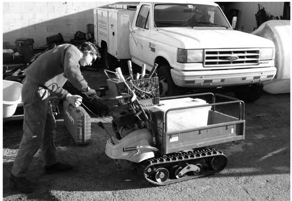
Motorized wheelbarrow that Shelterbelt uses to get tools and supplies to remote work sites.
