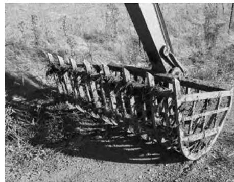
This skeleton basket strains the vegetation before loading it onto a truck for removal.
