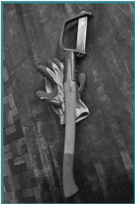
The Swedish Brush Axe is used for clearing brush and is much safer than a machete. Photo: Ken Moore
