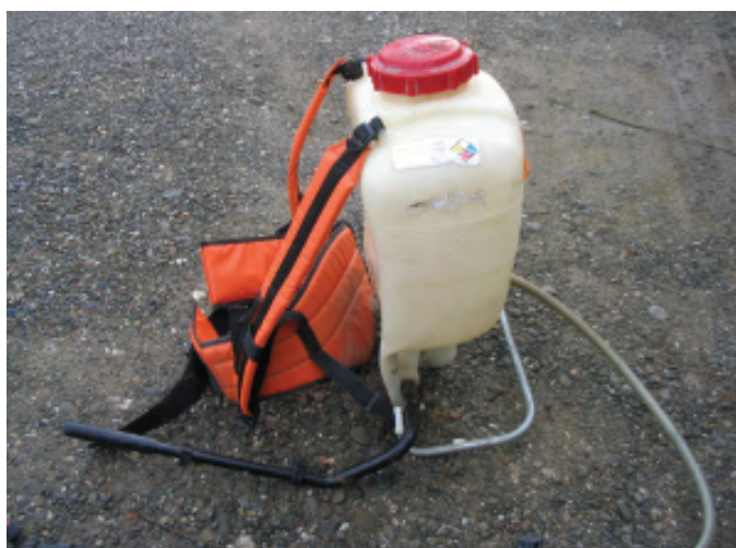
Backpack spray rig. A hand-pumped sprayer can be an economical way to treat small patches, such as spot treatments in a follow-up program. (Photo: G. Kyser)
