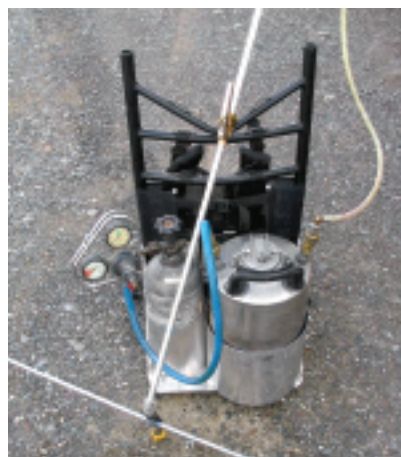
CO 2 sprayer. A backpack sprayer using compressed CO 2 can be used with a spray boom for broadcast treatments, or for spot treating at a distance of 20 feet with a focused nozzle spray. (Photo: G. Kyser)
