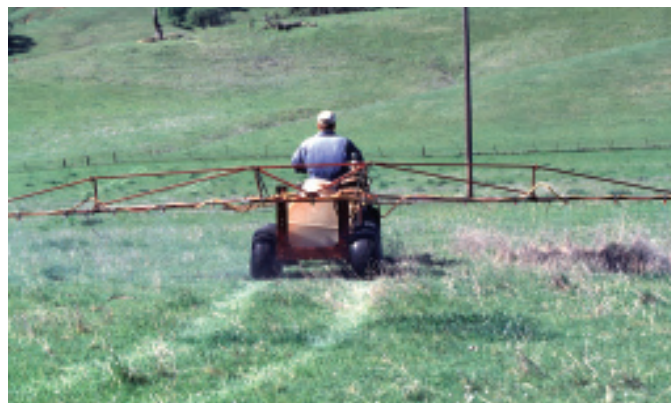
Treatment from an ATV. Application of herbicide for yellow starthistle control in rangeland can be made using a boom mounted on an ATV.
