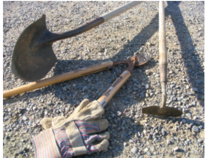
Hand tools. Shovels, lopper, and hoes are effective for small, sparsely-spaced populations. (Photo: G. Kyser)
