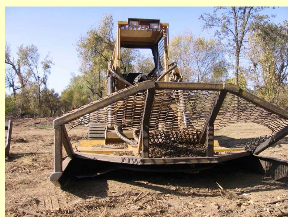
Figure 4: After goats reduced biomass, a mechanical masticator was used for final clearing
