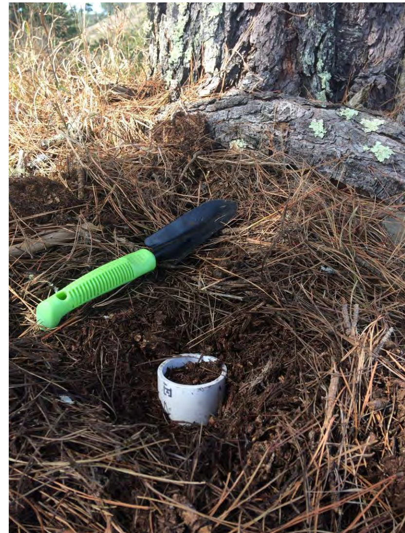
In situ N mineralization cores
