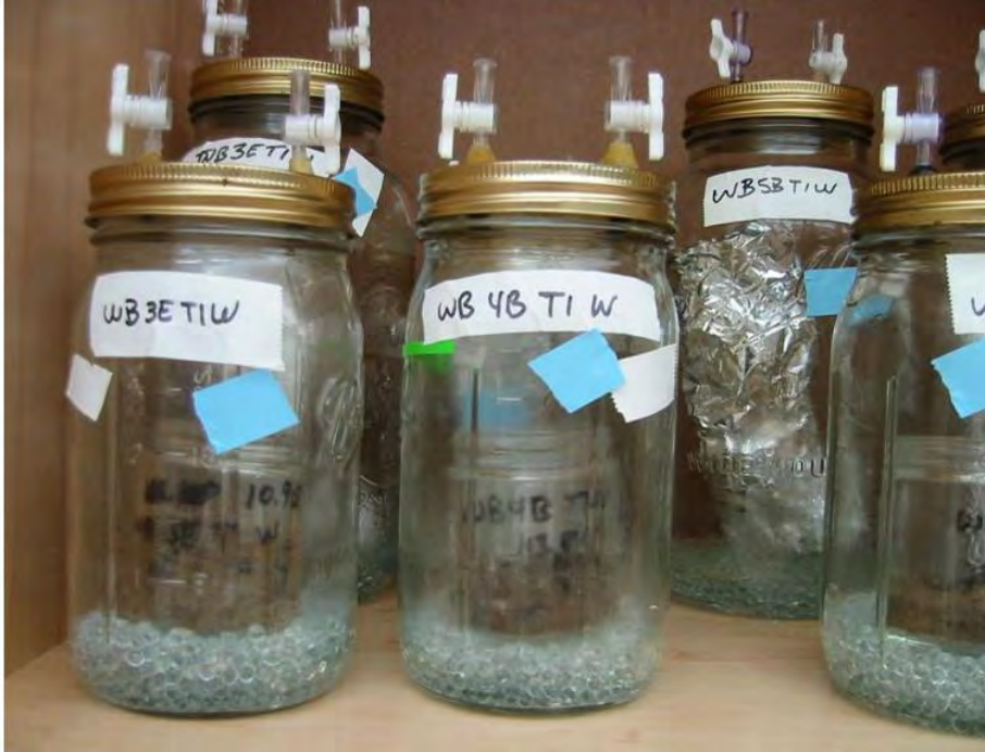
C mineralization: measure heterotrophic respiration by rate of CO 2 efflux
