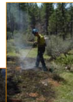
Figure 3. Flaming treatments were conducted with Weed Dragon™ backpack propane torches (100,000 BTU)
