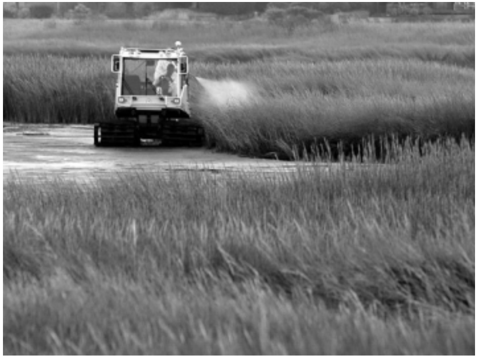
A MarshMog treats invasive Spartina along the edge of a marsh in the San Francisco Estuary. The vehicle is designed to drive on soft surfaces with minimal disruption. Photo: Drew Kerr.
