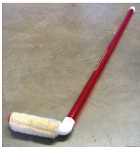
“Hockey stick” wick applicator. A rope wick is an alternative to spot spraying and reduces the likelihood of herbicide drift. (Photo: G. Kyser)
