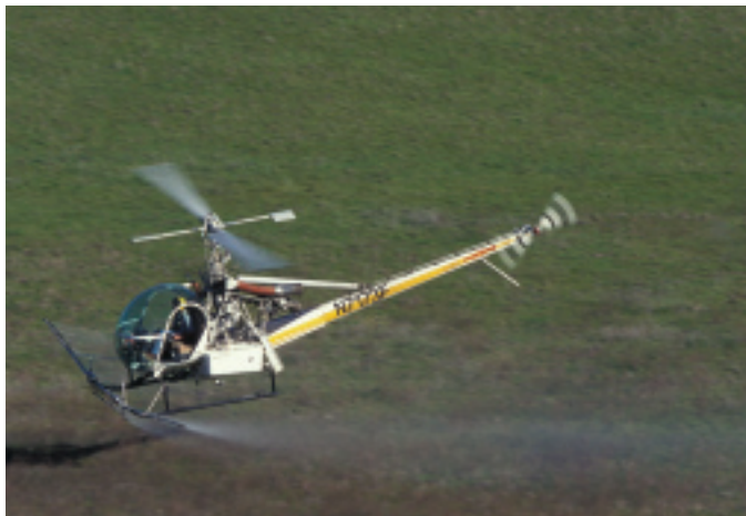
Helicopter spraying. Helicopter application can be used for large infestations but care must be taken to reduce drift. (Photo: J. Clark)
